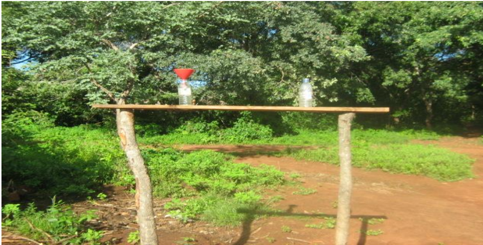
Figure 7: Rain gauge in Sikwenda village
